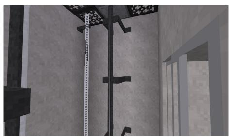
Install magnets on the tape above the top of the door at each landing. Brackets are available for supporting the ends of the tape.
